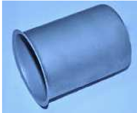
Figure 17: Successful Cup Drawn with Trial 1 Conditions
